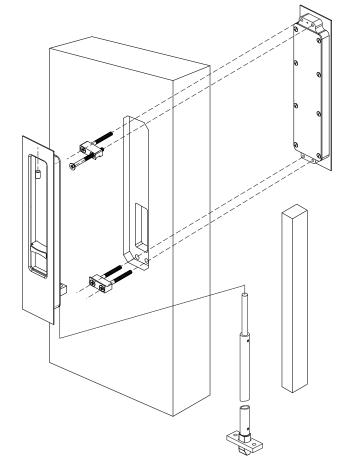
For painted timber doors the rod recess channel is machined into the door surface. Once the rod channel is created a timber insert must be packed into the cavity (leaving the rod channel clear) and the door must be refinished for painting.
