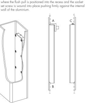
The inside flush pull is then fastened as per the 'A' fixing method'
