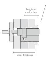
Remember to allow for the protrusion of the cylinder for the lever handle back plate – 12.5mm, or escutcheons -7mm or 9mm. Specify door thickness when ordering this product. Refer chant™ Escutcheons in Accessories Section for thickness.
