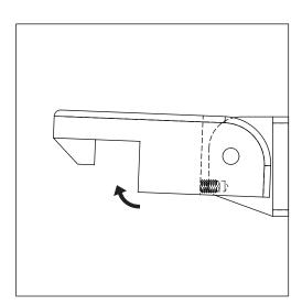
Adjustment screw will allow you to increase the angle of t he Hold Back to the mounting piece, suitable for the linear board.
