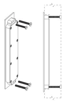
The Flush Pull is back fixed from the inside of the door. This fixing can be used for single installation or installing two types of different flush pull types back to back, eg order the external pull 'R' fix and the internal pull 'B' fix.
