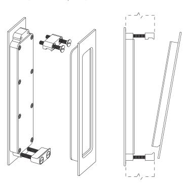
The outside Flush Pull is back fixed with mounting screws that pass through the mounting blocks on the inside of the door. The inside Flush Pull is inserted into mounting blocks then fastened with a socket set screw at the top of the finger recess.
