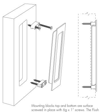
Pull is inserted into the mounting blocks, then fastened with a socket screw at the top of the recess.
