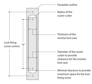
"X" is the height setting, to be set on the crank arm on the lock mortising machine. Dimension "X" is approximately 5-10mm ( $\frac{3}{16}$ " -  $\frac{3}{8}$ ") less than the height of the lock case in most situations. It is recommended to trial mortise, trial fit the lock, adjust and remortise the door if the lock does not fit.
