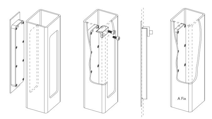
Back to back fixed. Essential where fixing security of the outside fush pull is required. The outside pull is fixed from the inside of the stile with screws and a clamp block. The inside flush pull is then fastened as per the 'A' fixing method'. All locking flush pull systems utilise this configuration as standard.
