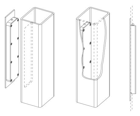
Surface fix, single side. The flush pull hooks into the aluminium at the bottom and is fastened by a socket set screw at the top of the pocket against the aluminium wall.
