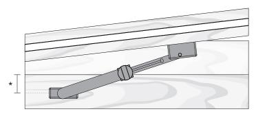
$\bigstar$  Adjust this dimension to fasten to solid timber away from the weather seal groove if applicable.
